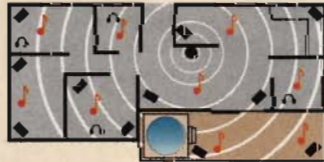
Recoton's transmitter sends music through walls to wireless speakers over a 75,000 square foot area.
