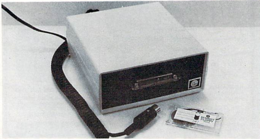
The Exatron Stringy Floppy, with a wafer inserted in the front slot.
