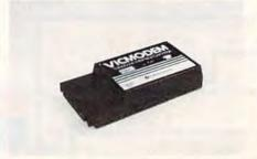
The VICmodem is an example of a directconnect modem – it bypasses the telephone handset.
