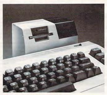
The Unitronics Waferdrive Module, a low-cost mass storage device for the VIC and 64.
