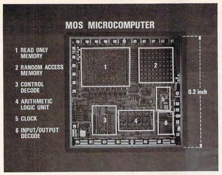
An average chip is only .2 inches (1/5 of an inch) on a side. Yet it is made up of several complicated parts including a part that does arithmetic (#4 – Arithmetic Logic Unit), a "clock" (#5), a "brain" (#3, #4, #5, and #6 working together), and two kinds of memory (#1 and #2).
