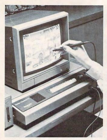
Drawing pictures directly on the TV screen with a light pen. (Courtesy of Matsushita Electric.)
