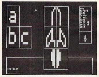
You can build complicated shapes by combining simple, rectangular building blocks or special graphics characters. Shown are three letters of the alphabet and a rocket. When the rocket is reduced, it becomes much more realistic. (Photo by Alice Collette. Courtesy of Rosetta Inc. Reprinted from Small Computers with permission of the publisher, Franklin Watts.)
