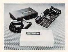
The Interpod, an intelligent freestanding interface for the VIC and 64, uses a 6502 to communicate with all Commodore and RS-232 devices.
