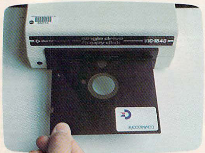
The proper way to insert a floppy diskette — holding it by the edge (face up with the notch on the left) and sliding it into the slot.
