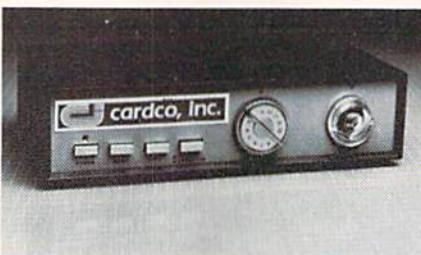
Cardco's MT/2 monitor tuner converts a computer monitor into a TV.
