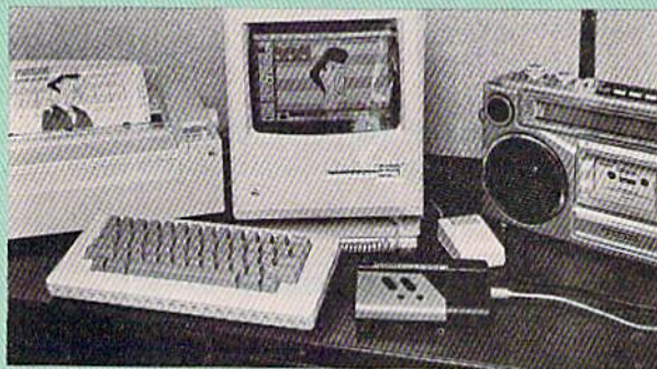
The Shuttle Communicator can download information from a radio station to any home computer, at speeds of up to 4800 baud.
