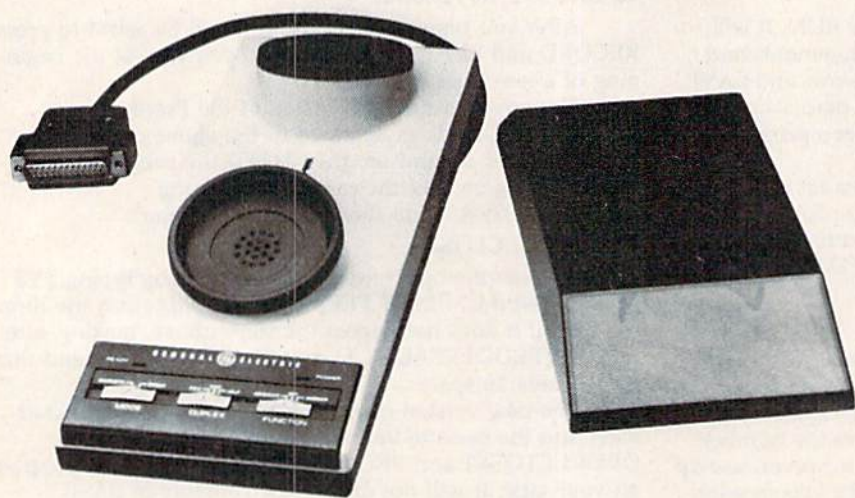
One member of General Electric's new family of computer peripherals is this combination acoustic/direct-connect modem.
