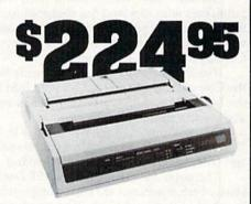
Features include mode selection, pitch selection, 180 cps in high speed draft mode and 120cps in utility mode. Near-letter-quality text prints at 30cps. Includes both friction feed and fixed tractor for standard width perforated edge. Both Commodore and standard parallel input.
