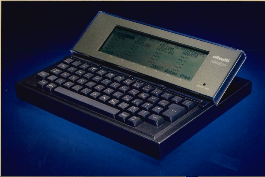
The new Olivetti M-10 portable computer features a tilt-up screen
