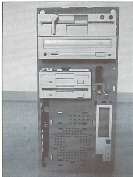
Front view of the hYbriD 1. The recess at the lower left side for the C64 motherboard is clearly seen
