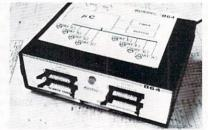
BUSSter modules are available in several digital and analog configurations. The internal buffer and timer provide flexibility by allowing the BUSSter to collect data while the host computer is busy with other tasks.
