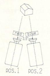
the red filter (position 1). Move the camera about  $2^{-1/2}$ " to the right (or rotate the object <u>slightly</u> to the left) keeping the camera aimed at the center of the object. Now scan the blue plane with the blue filter (position 2). Next, view the object in color, (4096-color mode works best): you will see a double-image with blue and red 'coronas' to the left and right.
