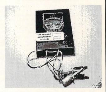
On-Target drive alignment meter.
