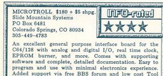
Here's a very big idea from a small and relatively unknown company. The Microtroll, from Slide Mountain Systems, was designed as a general purpose interface board for the Commodore 64. The Microtroll allows designing and constructing custom microcomputer controllers, monitors, and data acquisition systems with very little additional work. It also gives students, hackers and hobbyists the capability to learn about these systems firsthand and experiment with what they can do.
