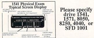
**Package includes:** • True digital alignment disk with offset tracks. • Mechanical Stop Test • Speed test • Illustrated manual with instructions for performing alignment, adjusting speed and stop position. • Hard copy mode to print test results for future reference.
