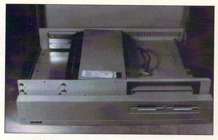
Inside view of the *Arrow 1500* with the flip top up and the faceplate down. Expansion slots are to the left, power supply is down the center, and the drive plate is to the right.
