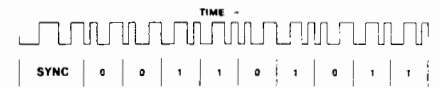
Figure 2. Example of tape format for a single byte. The SYNC bit is followed by 8 data bits with the least significant bit first. The value of this byte is thus $AC in hex. The last bit on the right is the parity bit. Since in this case the number of "1" bits is even, the parity is even, so the parity bit is "1". The parity bit helps to check for errors.
