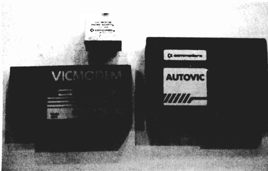
Three components comprising the VIC modem, phone adapter and auto-answer system.
