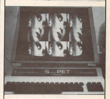
This is a graphics board which is universally compatible with all models of PET's. With Superpets (both 2 and 3 boards) It works equally well on both the 6502 and 6809 side as well as with OS-9.
