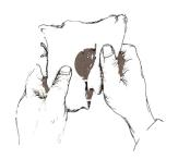
To remove any dirt or dust from the ball area, just blow gently into the opening. Around the top of the opening, there are three metal rollers. To clean these, take a cotton-tipped
