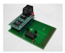
The FB-NET cartridge is a new Ethernet adaptor for the c64/128 thats compatible with both the RRNET and TFE (The Final Ethernet). The FB-NET includes and Olimex CS8900a-h header board and two jumpers used to set any of the following I/O addresses: \$DE00, \$DE08, \$DF00, \$DF08 The Olimex CS8900a-h board is soldered onto the to FB-NET cartridge board. For more information about the Olimex CS8900a-h please refer to. http://www.olimex.com/dev/cx8900a-h.html
