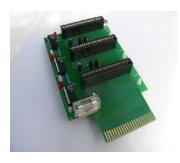
The FB-3XP is possibly one of the most versatile 3-slot cartridge expanders that supports the following features: Fuse protection to prevent accidental damage of the c64/128 computer.. - High quality ROHS compliant components with gold edge contacts. - Mini push button reset switch. - Electrolytic capacitors ensuring reliable power to each cartridge slot. - Activity LED for each slot indicating when a cartridge is
