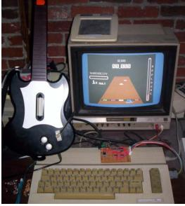
if a guitar controller is detected, it will encode strum up, strum down, lift up, and the whammy bar onto the two potentiometer lines of the joystick port. While this extra guitar functionality is usable by the Shredz64 (see above article) game only (and any future projects), the normal functionality of the PSX64 interface can be used with any game, and works well! Purchase a PSX64 interface from Synthetic Dreams at <u>http://www.synthdreams.com</u>
