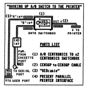
"GEOcable" may be purchased from Creative Micro Designs, Inc. for \$29 plus \$5 shipping. (1-800-638-3263). One good source for the switch box and connecting cable would be JDR Microdevices, (1-800-538-5000). The Data Switchbox (#RSP-2) is only \$9.95 and the six foot CEN36P to CEN36P cable (#CBL-CNT-MM) runs \$14.95. Shipping is about \$5 for the two items.
