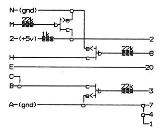
Though there are no known reports of this circuit not working, the FAQ notes that should problems be experienced, try reversing the clock signal by reconfiguring the circuit as follows. Connect the collector on the middle transistor to pin 2 of the user port, connect the emitter to pin H, and connect a 1K ohm resistor between pin H and pin N or A.
