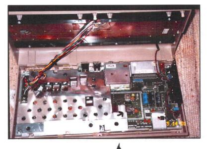
Note a small black arrow pointing to the chip in U19 that had the heat sink attached.
