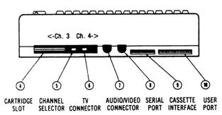
4. Cartridge Slot. The rectangular slot to the left
