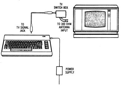
The C64 is now correctly connected, No additional connections are required to use the computer with your TV. The antenna switchbox will connect the computer to the TV when the slide switch is in the "computer" position. When the switch is in the TY position your set will operate normally.
