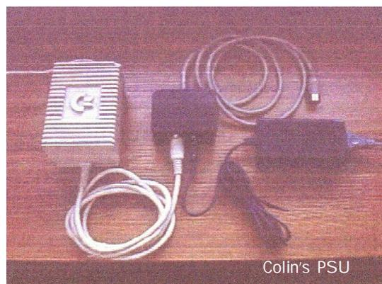
supply for your CMD Hard Drive. This PSU has the same pin out configuration and power supply as the **1541-II**, **1581** and the **Mk1 RAMLink**. This enables us to replace those old PSU's with a modern unit that is also repairable.
