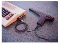
instructions include pinout information for the adaptor and a BASIC demo/test program for the LightPen mode. Note that only Control Port#1 on the C64 is connected to the Light Pen input on the VIC chip. Standard Light Pen software will also work with the Light Phaser.
