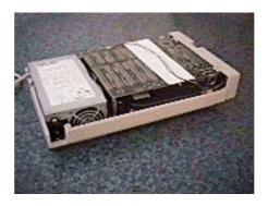
**Figure 2** - It is a very tight installation but with the correct PCB you can fit the FDD, HDD and PSU.
