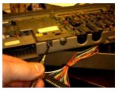
first! Tune your TV to a suitable channel then slowly turn the modulator screw and note the best position on TV.
