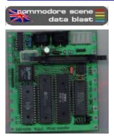
**DATA** : Need a 1581 but can't get hold of one - how about this ? Version 0.1.0 of the **DCN-2692**, which is a controller board that works like the CBM-1581.
