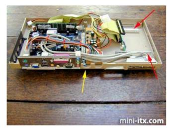
I decided to play around a little bit with the cables just to make sure they had sufficient length, the final arrangement would become a little tidier as you will see later on. A 256 MB RAM module was fitted since I think that it is the minimum (but also sufficient) amount needed to be able to work with XP Professional smoothly.
