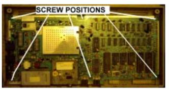
Once the Motherboard is removed place it on a flat surface where it won't get damaged. Now the outer casing of your machine can be washed and scrubbed with
