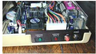
Cables were soldered on the leds and switches and plugged in the board. The original power led on top of the C64 casing was connected to the harddisk led output. That way the disk activity can be easily monitored.
