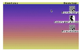
Here is the main Screen located on the right of the screen are three applications allowing us to access the disk directory, set the network configuration and also list the processes running. On the top menu pull down bar are items for Contiki and desktop. Under the Contiki pull down menu we have the following options.
