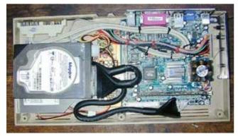
On the right side the original C64 metal lid can be seen. Normally this would house the power connector, power button and the two joystick ports. I converted it by glueing a piece of aluminum on the backside and drilled holes in it to contain two leds and two push button switches. The green led is lit when in "sleep mode", the red led is the "on/off" indicator. The red button is for resetting, the black one for powering up/down the system.
