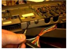
first! Tune your TV to a suitable channel then slowly turn the modulator screw and note the best position on TV.
