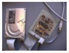
access an IDE hard device via the Commodore's normal disk drive serial port. Go to http://www.djupdal.org/ cbm/iecata/ to read about it. CS will cover this in a future issue.
