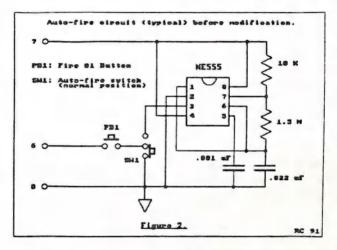
supply store, again) wired to form an OR gate. This prevents the ground provided by the "normal" fire button from being seen by the 555 timer.
