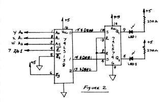
set up as two RS flip flops that latch the data. The set inputs of the 74LS74 are tied together and used for the reset input. The base address is set by I/O 1; if we hook the not enable line to I/O 2, the base address would be \$DFOO.
