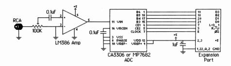
Figure 4: Schematic of the ZOUNDS! sound sampler. Use this newer one as it is suppose to produce cleaner sound samples.
