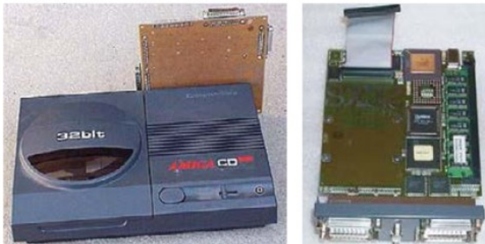
» Above left: These boards allowed developers to program games directly to the CD32 like a real Amiga. Right: The SX32 was one of a handful of devices to turn the CD32 into a full Amiga.
