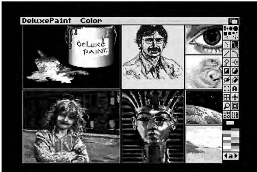
3.11 Eight images from earlier versions of Deluxe Paint, all originally with very different color palettes, combined into one using Deluxe Paint IV's HAM mode. The results are not perfect, but they are acceptable enough for many applications. Note also the gadget just below the color selection at the bottom right, indicating that this grid of 16 colors is just grid A of many grids available to the artist. However, because this grid represents the 16 primary HAM colors, they are the only ones guaranteed to show up with perfect fidelity when the artist uses them.
