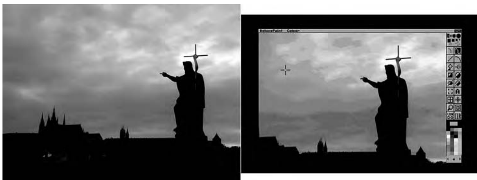
9.1 To the left is a true 24-bit image. To the right, the same image loaded into Deluxe Paint V's 256-color mode, with backing store enabled
