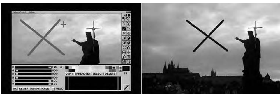
9.2 To the left, drawing onto a 24-bit image in Deluxe Paint V; to the right, the end result, displayed again in its full 24-bit glory. Color versions of these images are available on this book's Web site and may illustrate this example more clearly.
