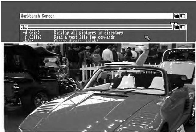
3.13 An Amiga display showing two radically different virtual screens on the same physical monitor screen. The AmigaOS Workbench screen at the top is 640 \times 200 resolution, with just four colors. The picture of the sports car is in overscanned 384 \times 480 resolution and HAM mode.
