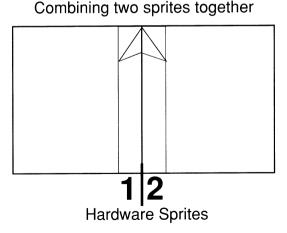
The maximum of eight hardware sprites therefore imposes a strict limit to the number of such objects you can display on a horizontal line. The total width of the objects must not
