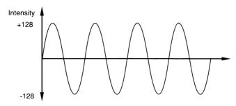
Adding several of these waves together, with different sizes and separate starting points, produces waves in the following pattern.
