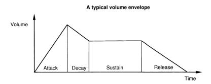
This sound is split up into four phases: Attack, decay, sustain and release.
