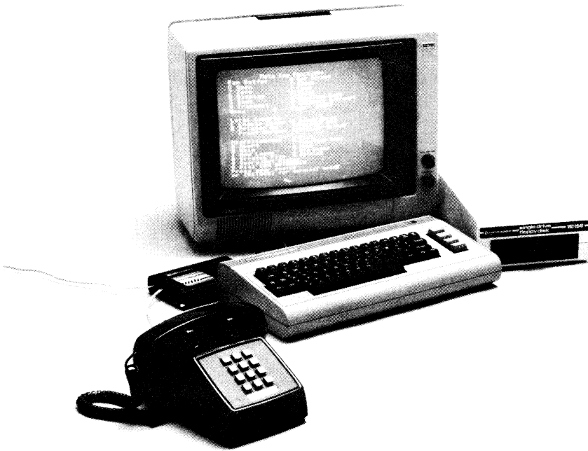
Figure 3-5. C-64 and Automodem telecommunications setup
