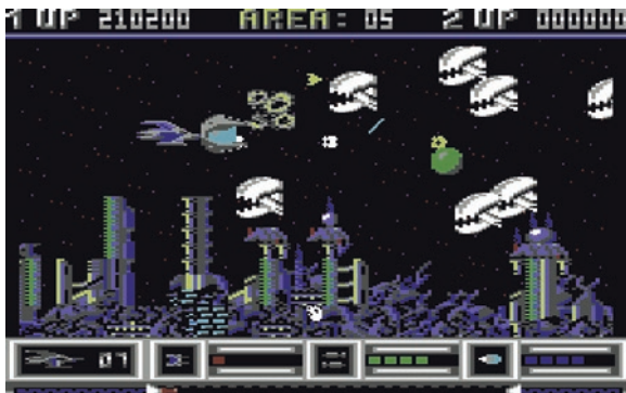
Fig. 2.4 Katakis, a graphically impressive space shooter released in 1989 by Rainbow Arts, used sprite multiplexing to the maximum effect, displaying many different sprites at once to create a frantic action experience
