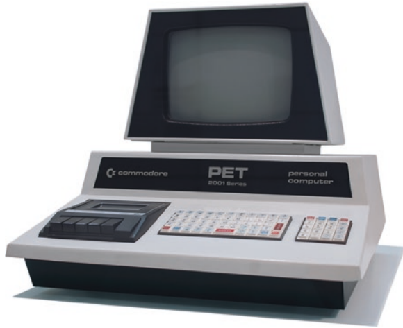
Fig. 1.3 The PET 2001: the first all-in-one personal computer. This figure is licensed under CC and copyright is owned by Tomislav Medak and Bill Bertram
