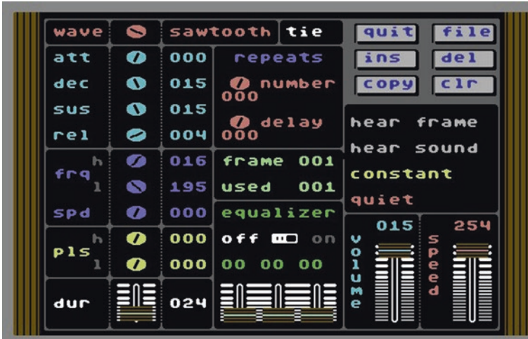
Fig. 5.6 The “Sound Maker” module that allowed easy access to the SID chip functionalities for shaping any in-game sound
