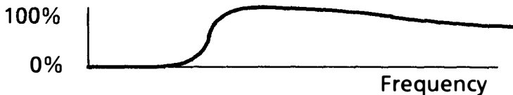
High-Pass and Band-Pass Filters Combined
